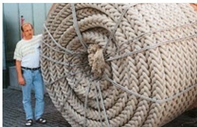
Complete rope cable, total weight approx. 2 t, rope diameter 16 cm
