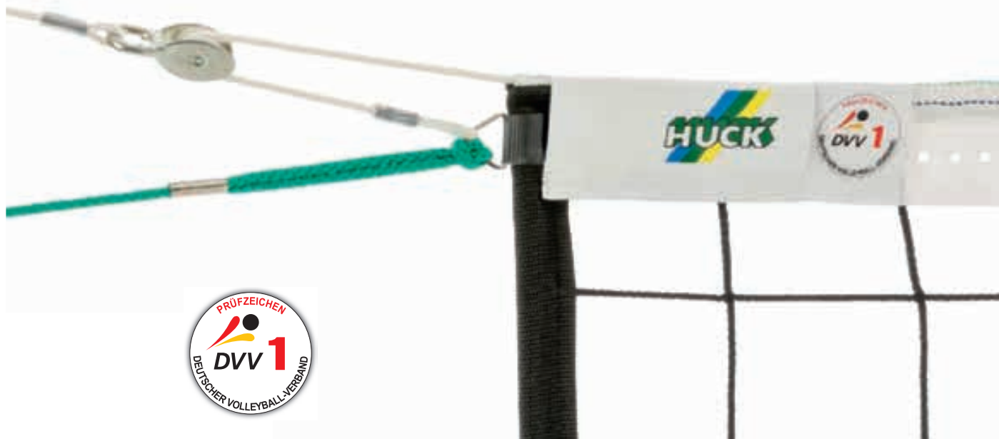
No. 5099: Volleyball Tournament DVV I competition nets. The pulley on each side of the net ensures a perfectly even tension over the entire area of the net.
