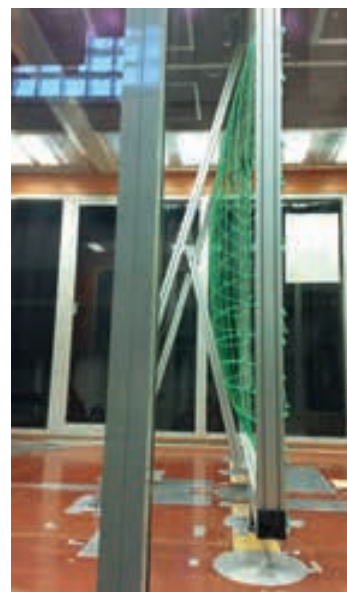
Test set-up to measure the wind load
